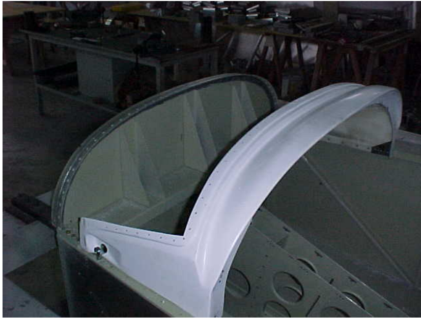
Figure 3.17: External view of 1 st section and firewall.
