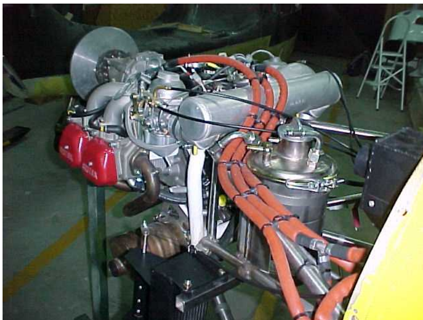
Figure 8.4: Rotax 914T installation 3.
