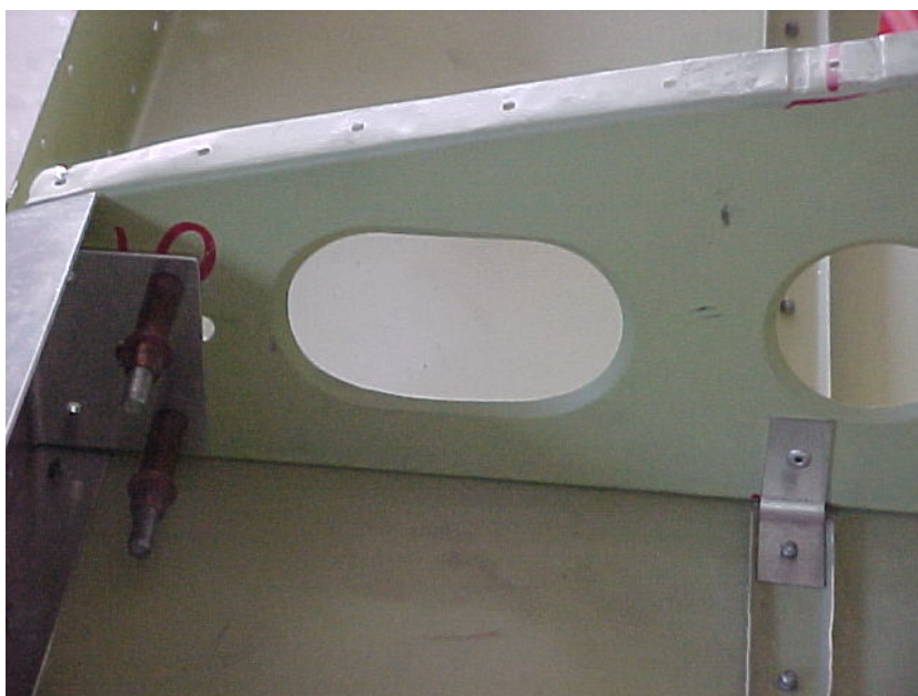
Figure 4.6: Wing tank reinforcement 2.
