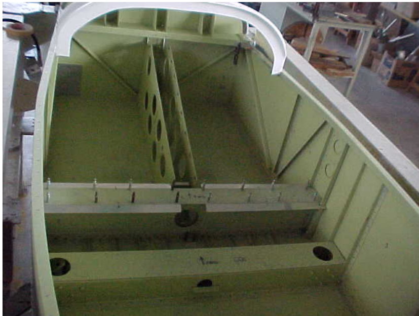
Figure 3.7: External view of the fuselage, 1 st section. It is easy to recognize the console, the wing box and the landing gear box.
