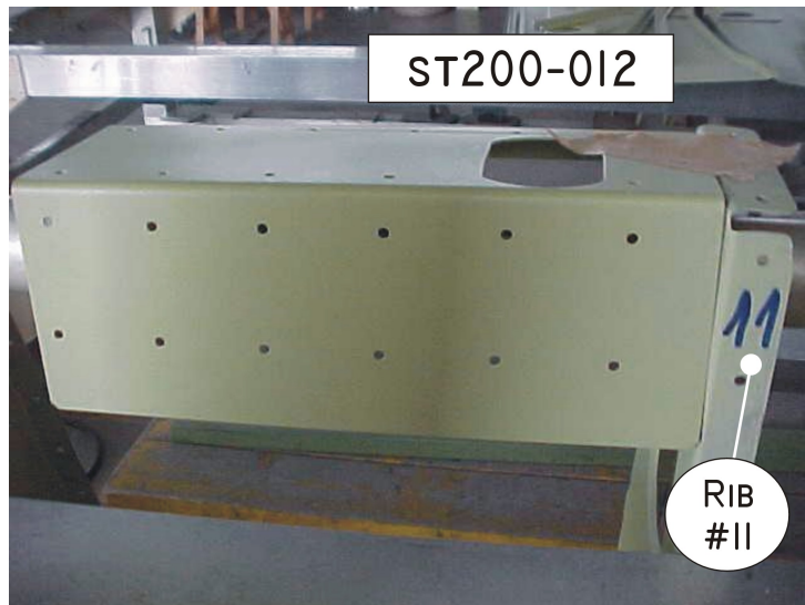
Figure 7.13: Hole for the aileron reinforcement rod. Such reinforcement is found to the inside of the wing rear spar ST200-012 element.
