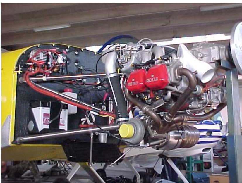
Figure 8.2: Rotax 914T installation 1.
