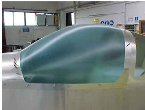
Figure 5.1: Canopy external covering.
