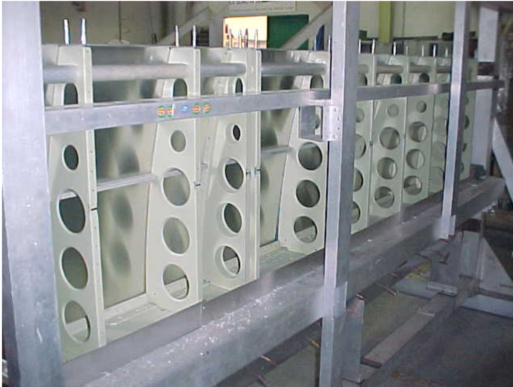
Figure 7.19: A clear scene of wing box assembling.
