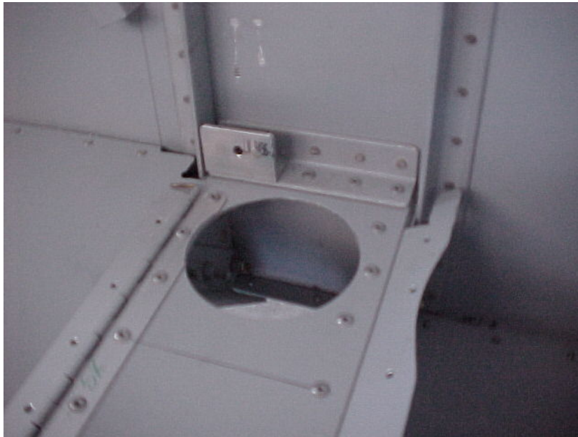
Figure 3.11: Detail of an angle on fuselage.
