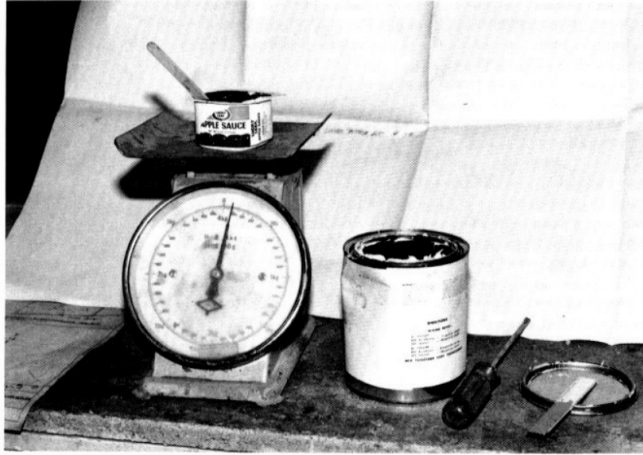
Here is the extent of the laboratory equipment used. A small Japanese household scale calibrated in grams, a small plastic container and two spatulas. One for dishing out the sealing compound and the other for the accelerator. Only small 100 gram batches were mixed at one time.
