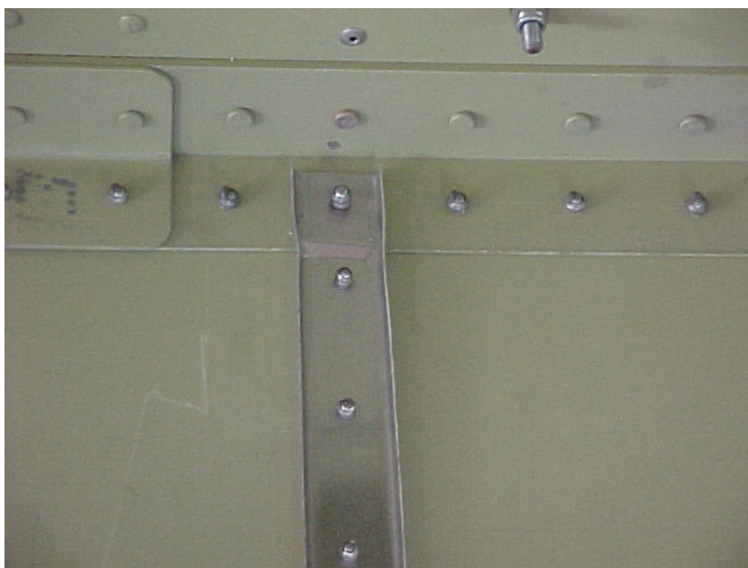
Figure 4.7: Wing tank reinforcement 3.
