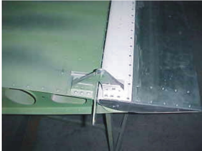
Figure 7.2: Flap breakdown (up) and flap hinge (down).
