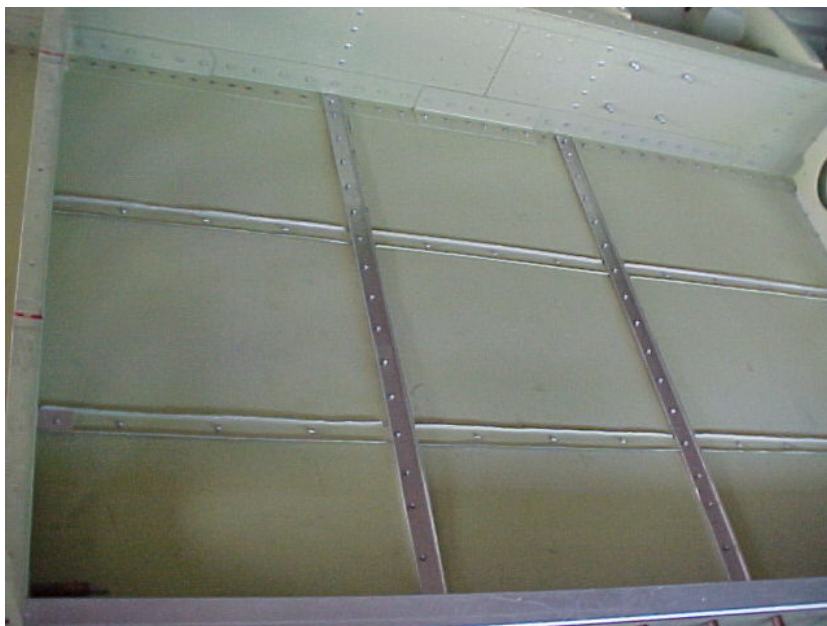
Figure 4.5: Wing tank reinforcement 1.
