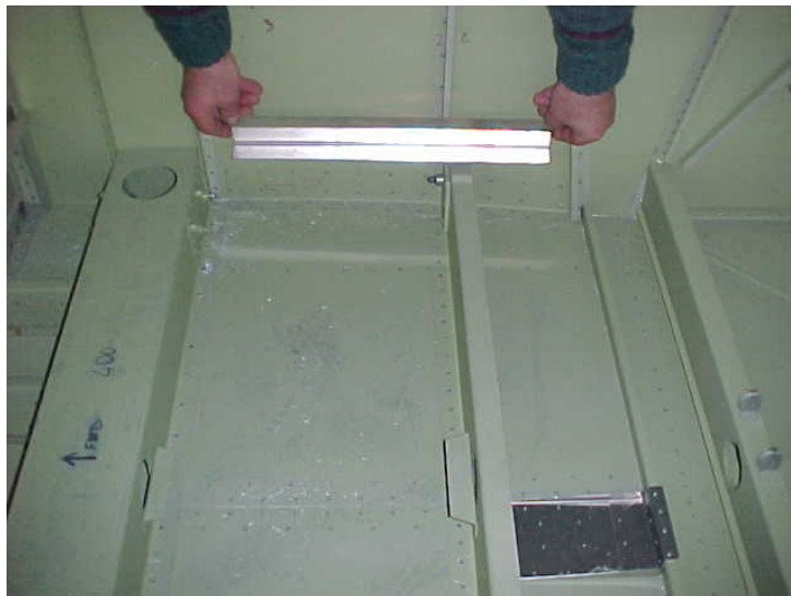
Figure 3.10: Fuselage rear beam.
