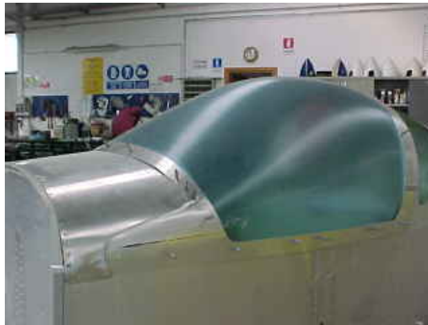
Figure 5.2: Canopy external covering.
