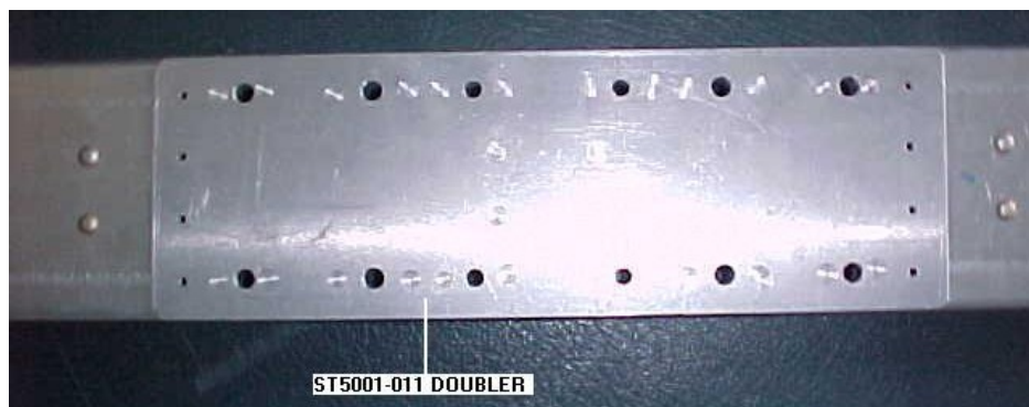
Figure 6.7: Stabilizer spar reinforcement.
