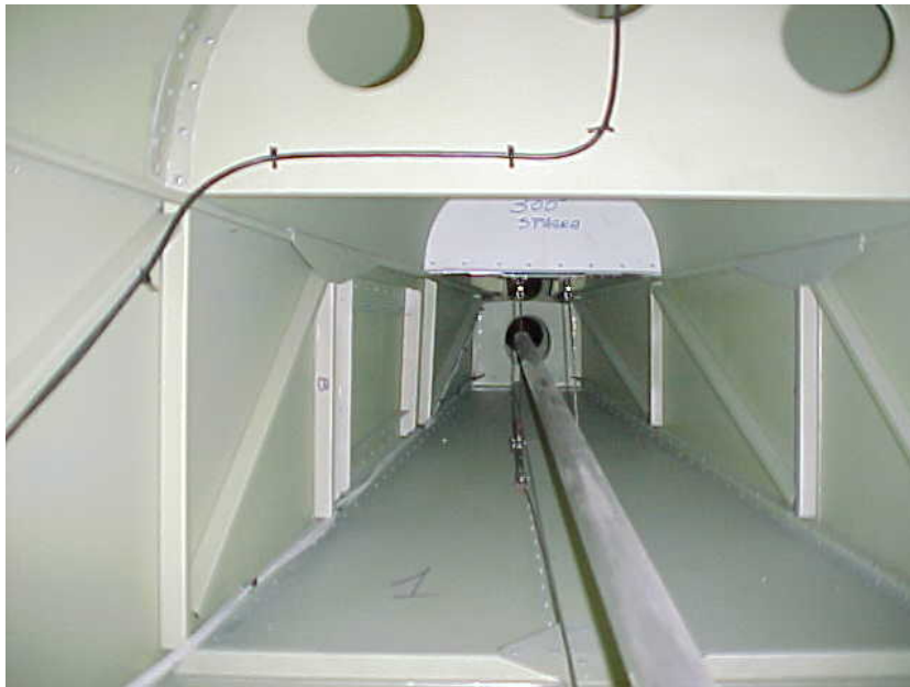
Figure 3.31: Fuselage 3 rd section: stabilizer control bar and rudder cable.
