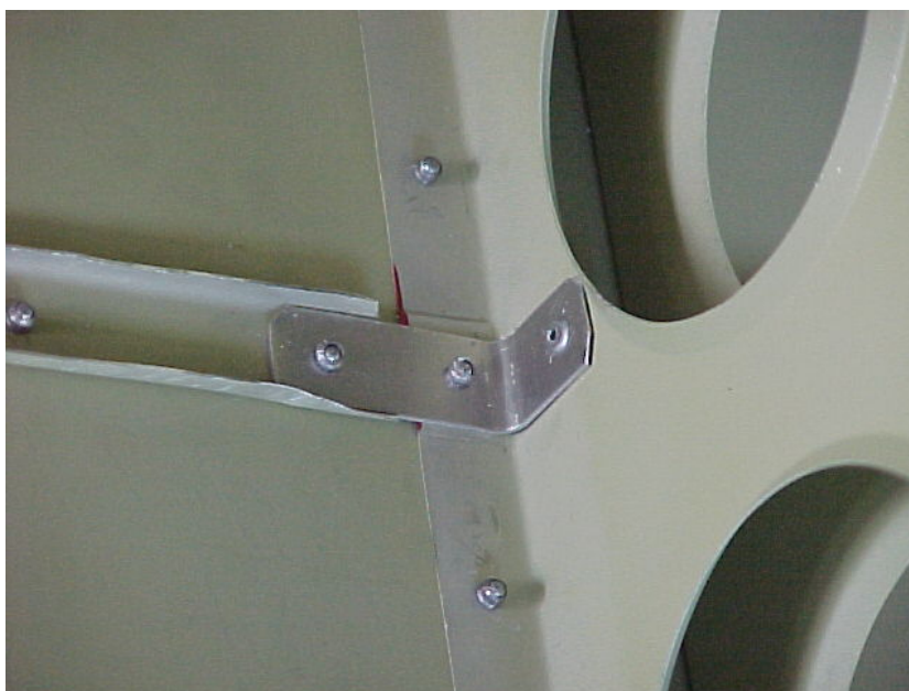
Figure 4.8: Wing tank reinforcement 4.
